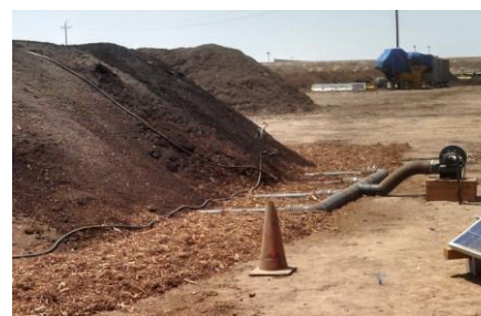
Aerated static piles
