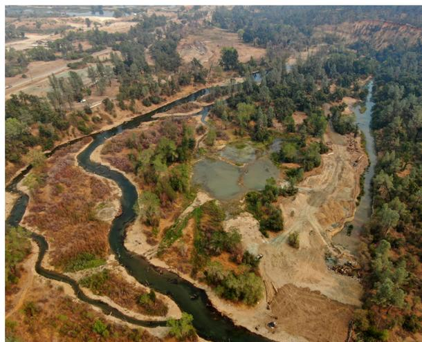
*A new stream channel created during the final stage of the [Lower Clear Creek Floodway Rehabilitation Project](#) provides islands, riffles, side channels and alcoves that improve fish habitat and fish passage. Credit: Aaron Martin/ Yurok Tribe Design Team*
